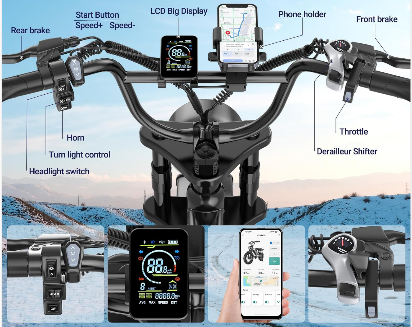
Image 5.1: Handlebar controls including LCD display, throttle, and switches.
