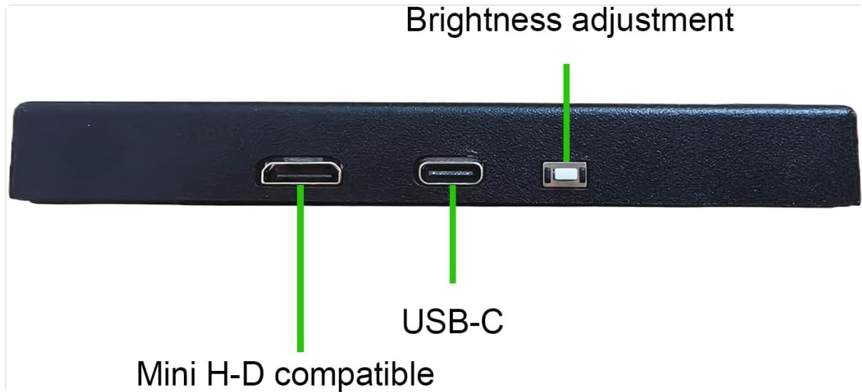
Image: Detailed view of the monitor's input and power ports, along with the brightness control.
