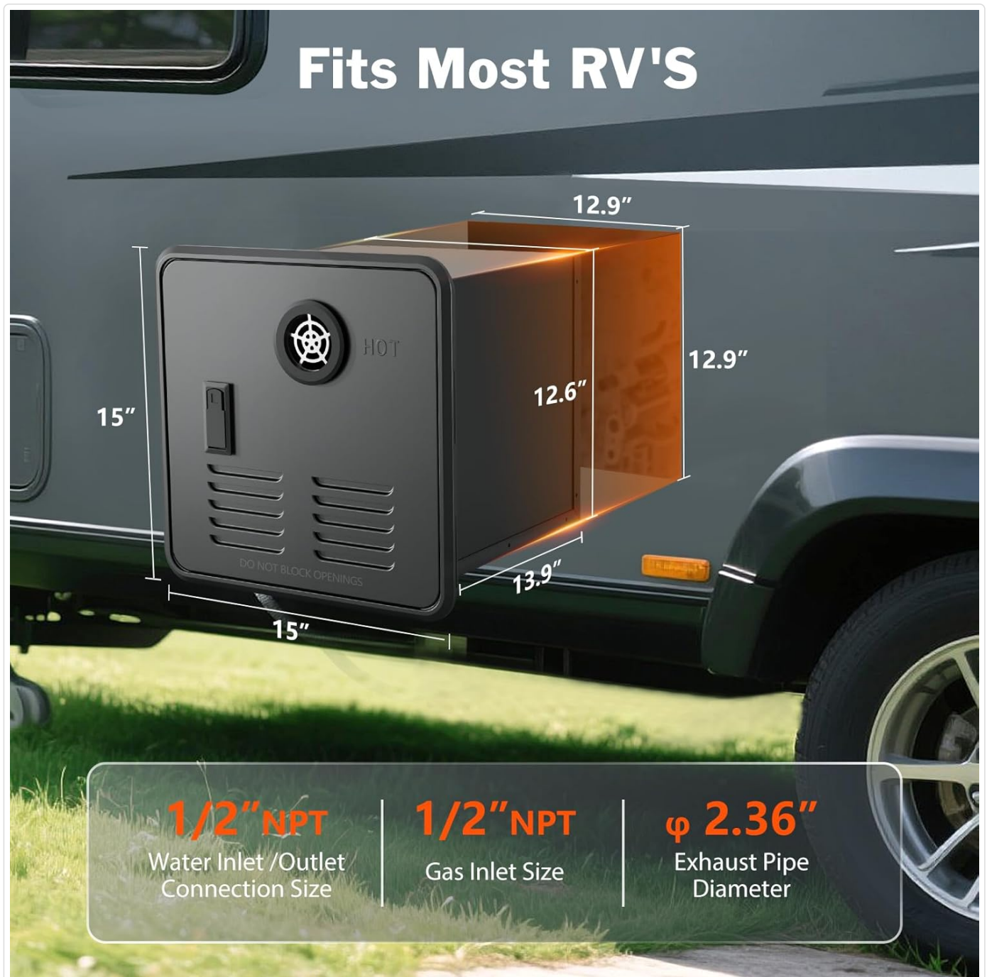
Figure 2: Installation Dimensions. The unit requires a 15" x 15" opening. The internal depth is approximately 12.6 inches. Water inlet/outlet and gas inlet connections are 1/2" NPT, and the exhaust pipe diameter is 2.36 inches.
