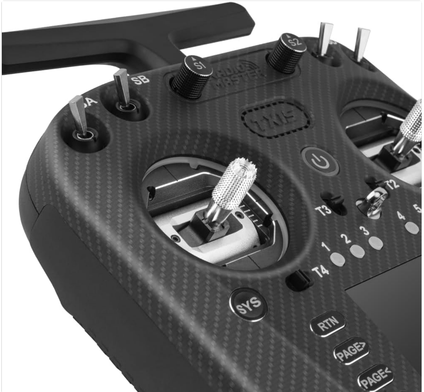
Image: Close-up view of one of the AG02 Hall sensor gimbals on the RadioMaster TX15 Max, showing its textured stick and surrounding controls.
