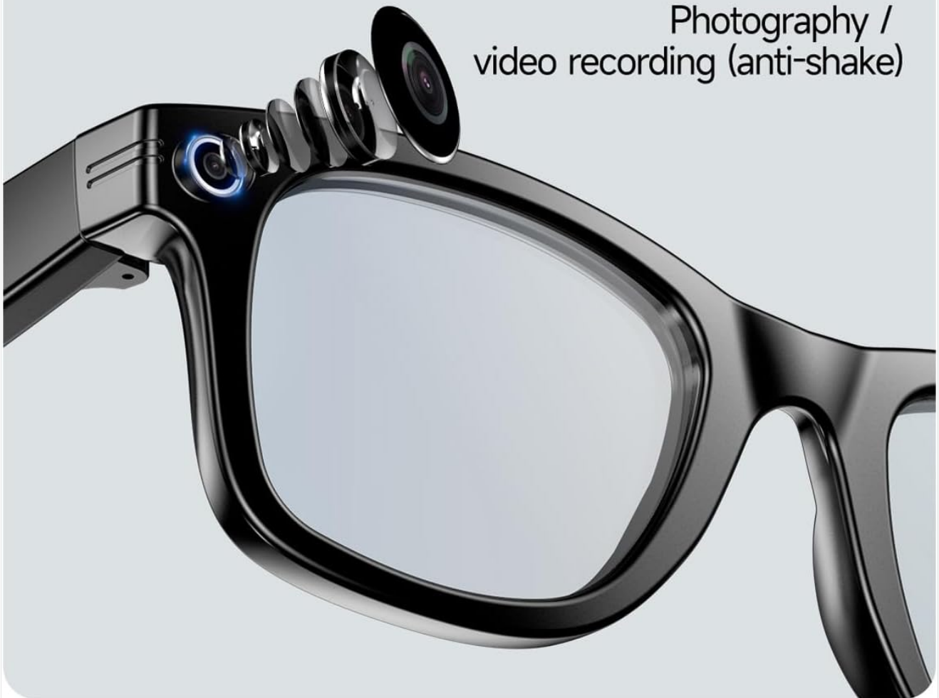
Figure 2.1: Detail of the integrated 800W HD camera on the smart glasses.
