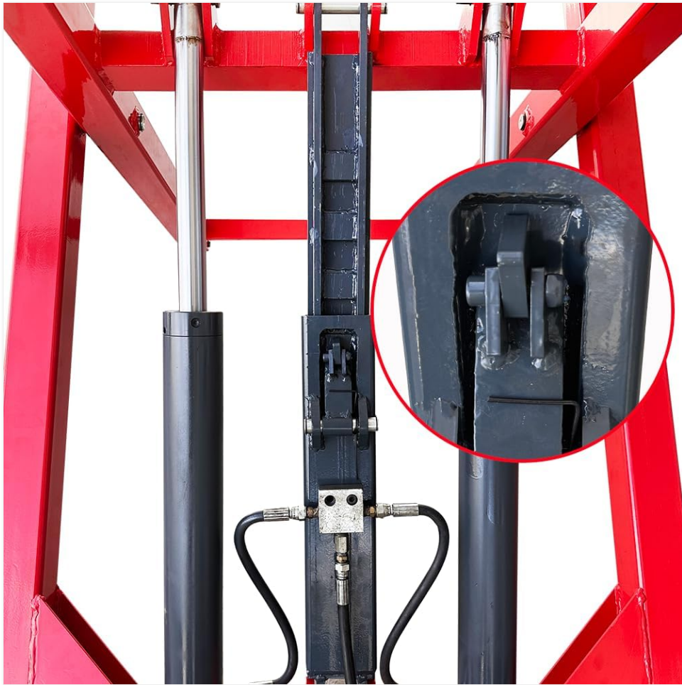
Figure 6.1: Detail of the mechanical safety locking mechanism, crucial for securing the lift at desired heights.
