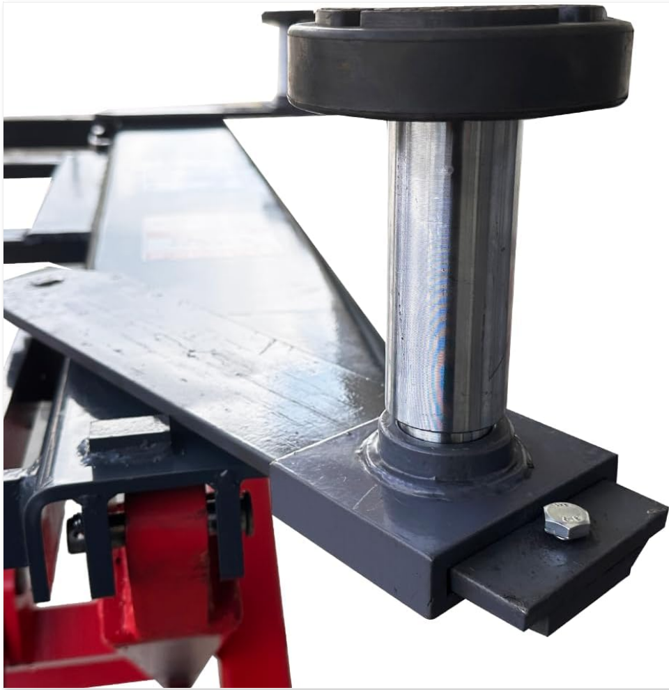
Figure 5.2: Detail of an adjustable lift pad, designed to accommodate various vehicle lifting points.
