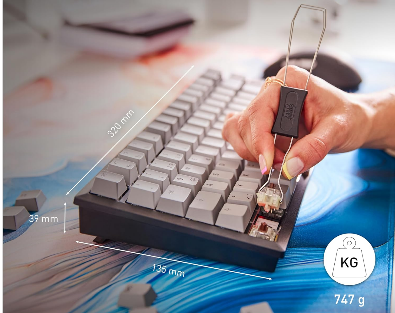
Figure 5: Demonstrating the hot-swap feature for replacing individual switches.
