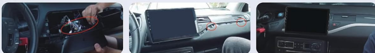
Image 3.2: Visual guide illustrating the disassembly process of the original car radio, showing tools and removal points.
