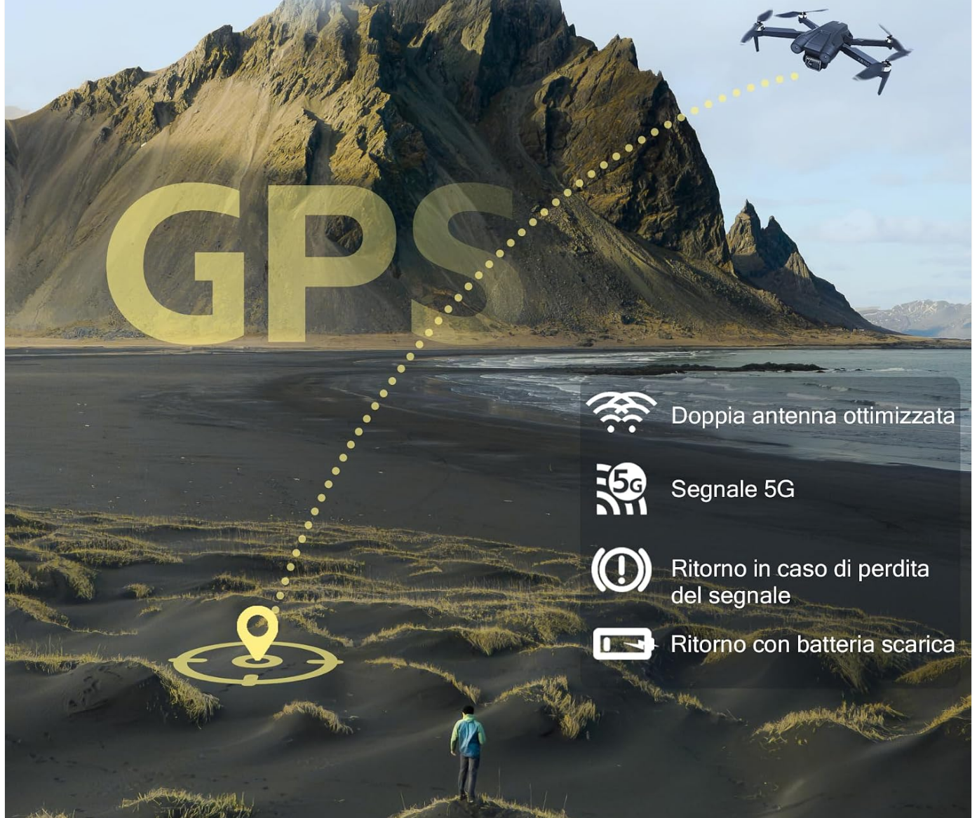
Figure 2: The GPS Smart Return feature reduces the risk of drone loss by automatically returning to the take-off point.
