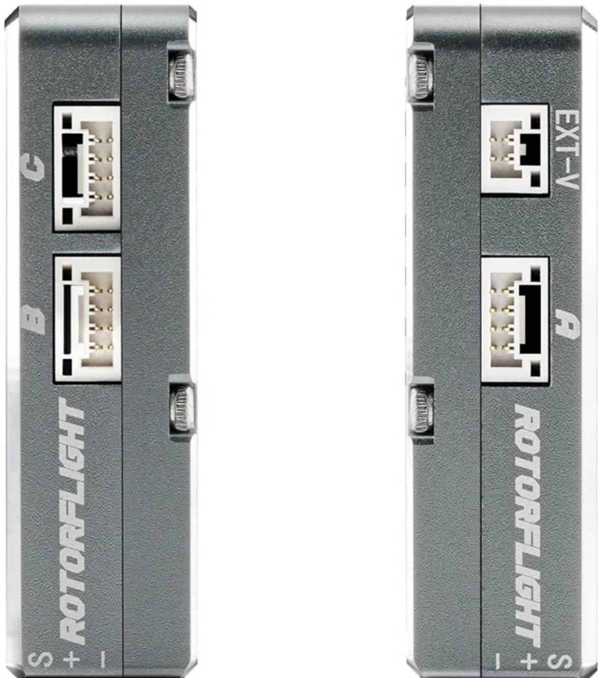
Figure 4: Side view illustrating UART ports A, B, C and EXT-V port.
