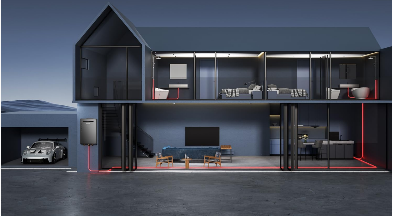
Image: Illustration showing the Ranein tankless water heater's suitability for single-family homes and townhouses, highlighting its 5.3 GPM, 130,000 BTU capacity for 3-5 points of use.
