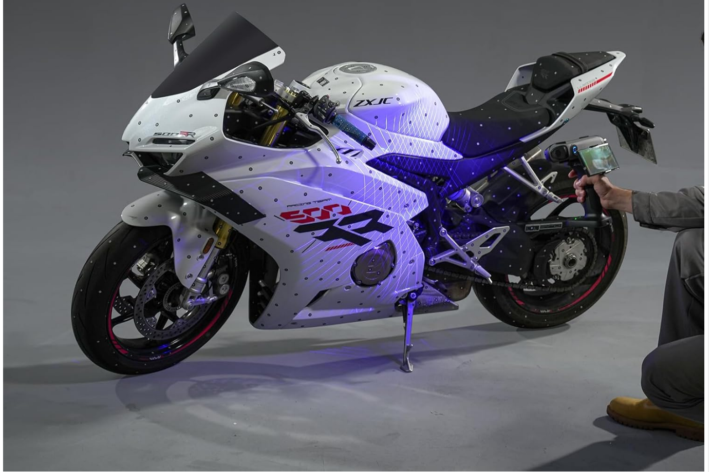
Figure 5: The scanner in use, demonstrating its high efficiency with 90FPS ultra-high speed scanning of a motorcycle.
