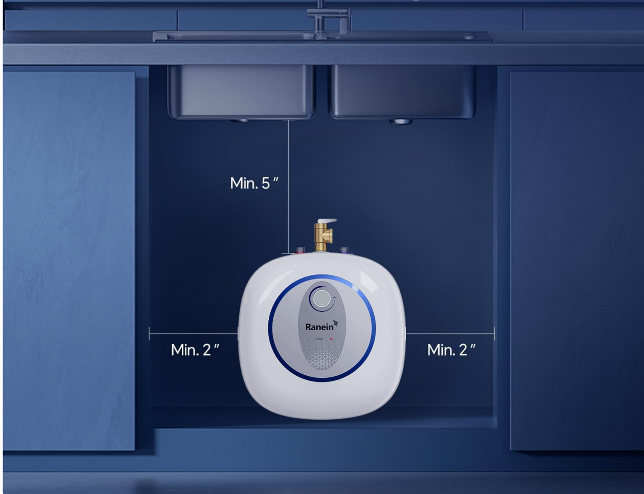
Image: Diagram showing minimum space requirements for under-sink installation, with 5 inches above and 2 inches on either side of the unit.
