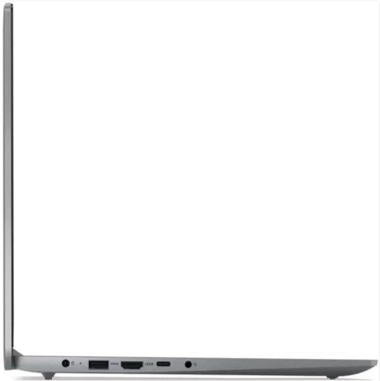
Image 3.1: Left side view of the laptop, illustrating the placement of the power input, USB ports, HDMI port, and USB-C port.
