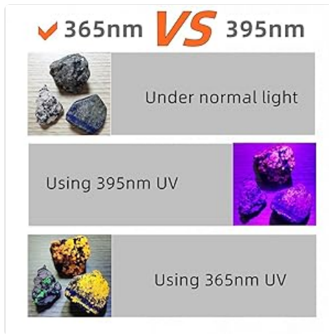
Image 6.2: A visual comparison of mineral samples under different lighting conditions: normal light, 395nm UV light, and 365nm UV light, highlighting the superior fluorescence activation with 365nm UV.
