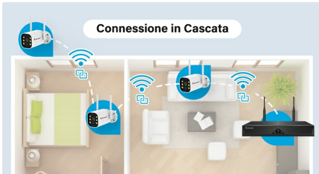
Figure 4: Cascade connection for extended WiFi range.
