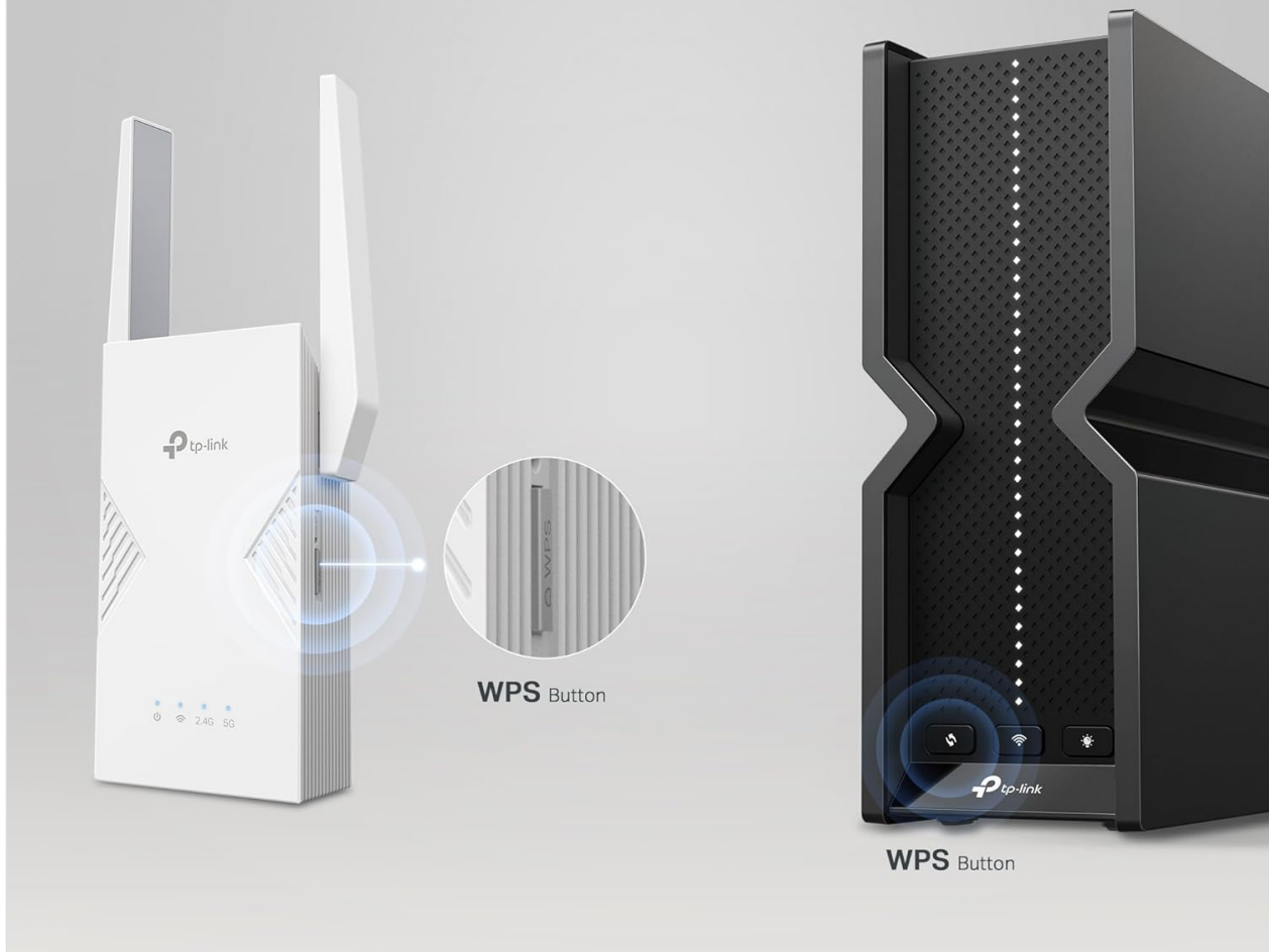
Image 2.2: Illustration of pressing the WPS button on both the router and the RE235BE.
