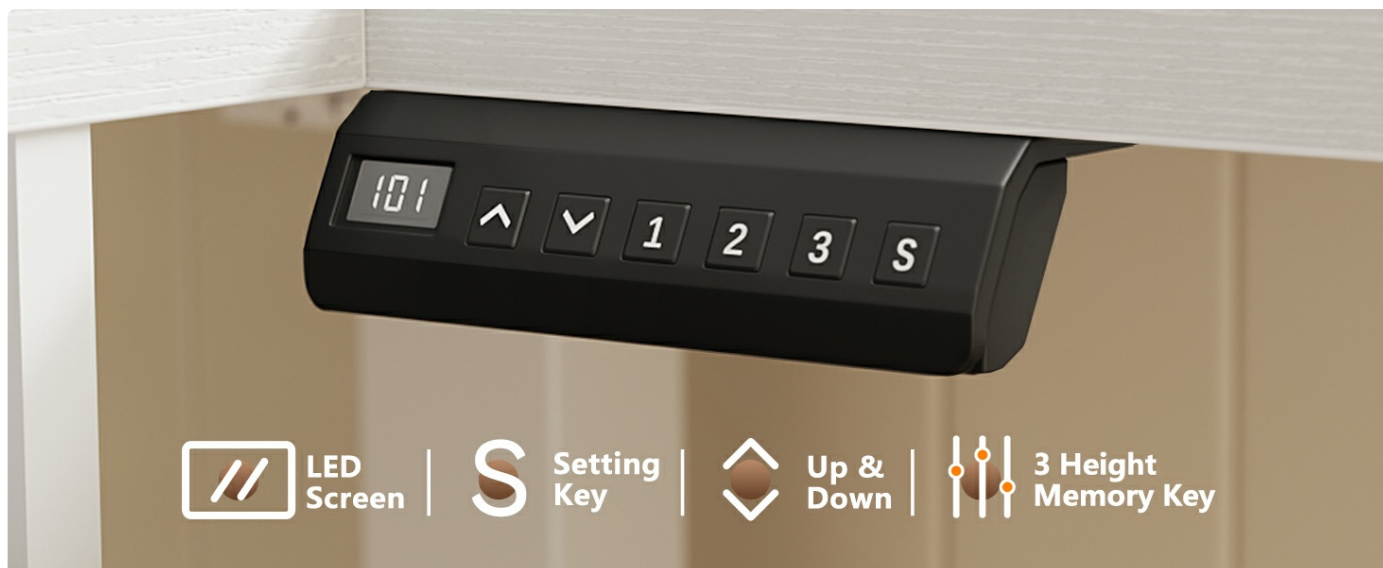
Image 3.2: A detailed view of the height adjustment control panel, featuring an LED screen, up and down arrows for manual adjustment, a setting key, and three programmable memory keys (1, 2, 3) to store your favorite desk heights.
