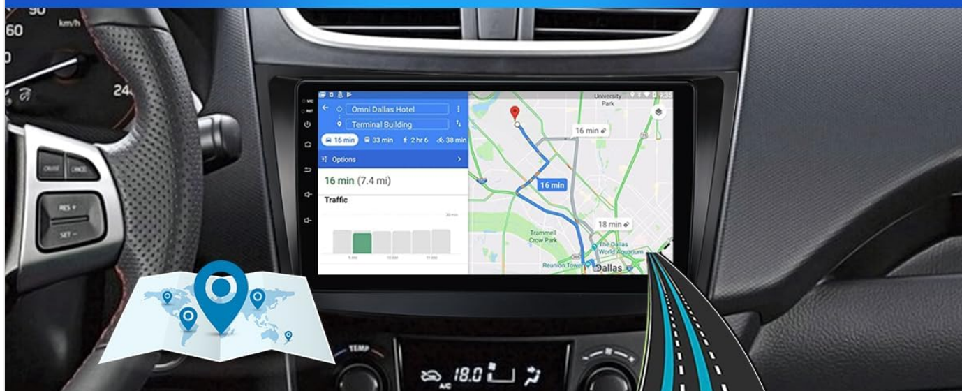
Figure 4.2: Navigation and Smartphone Integration. This image illustrates the GPS navigation interface alongside Apple CarPlay and Android Auto.
