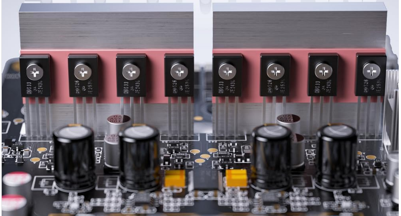
Figure 6: The discrete Class-AB amplifier circuit, designed for powerful and clean output.
