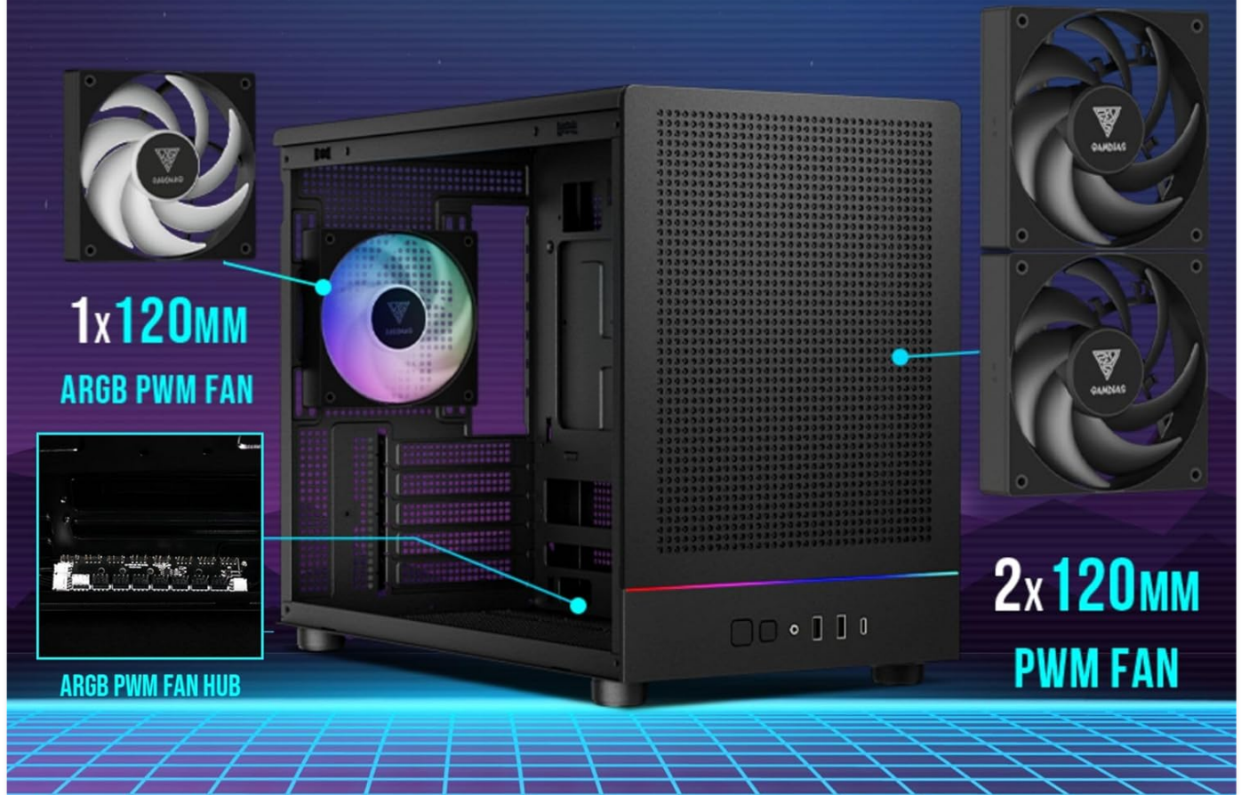
Image: Visual representation of the extensive airflow configuration, showing one 120mm ARGB PWM fan, two 120mm PWM fans, and an ARGB PWM fan hub.
