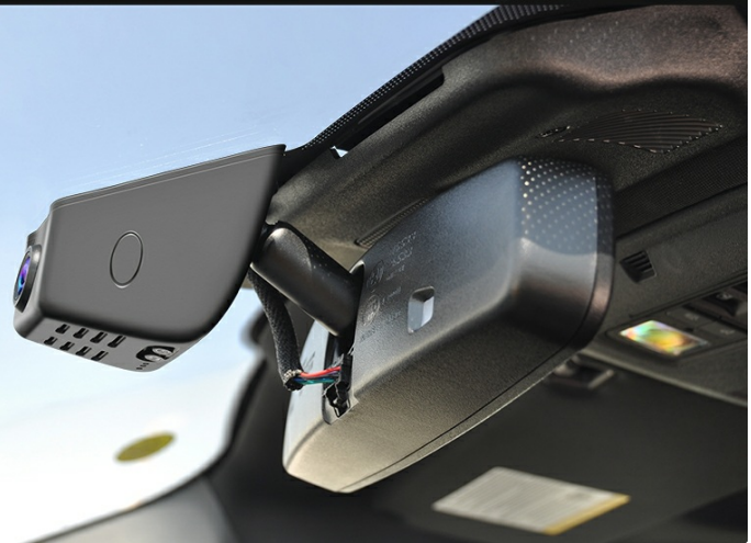
Figure 5: Key features for identifying Model A compatibility: screw, rearview mirror plug, and sensor cover.
