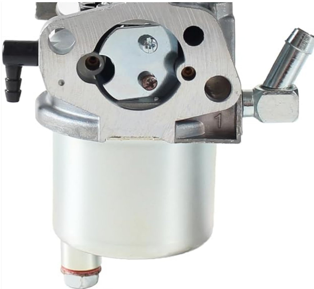
Image: Front view of the Pro Chaser carburetor, showing the air intake and mounting points.
