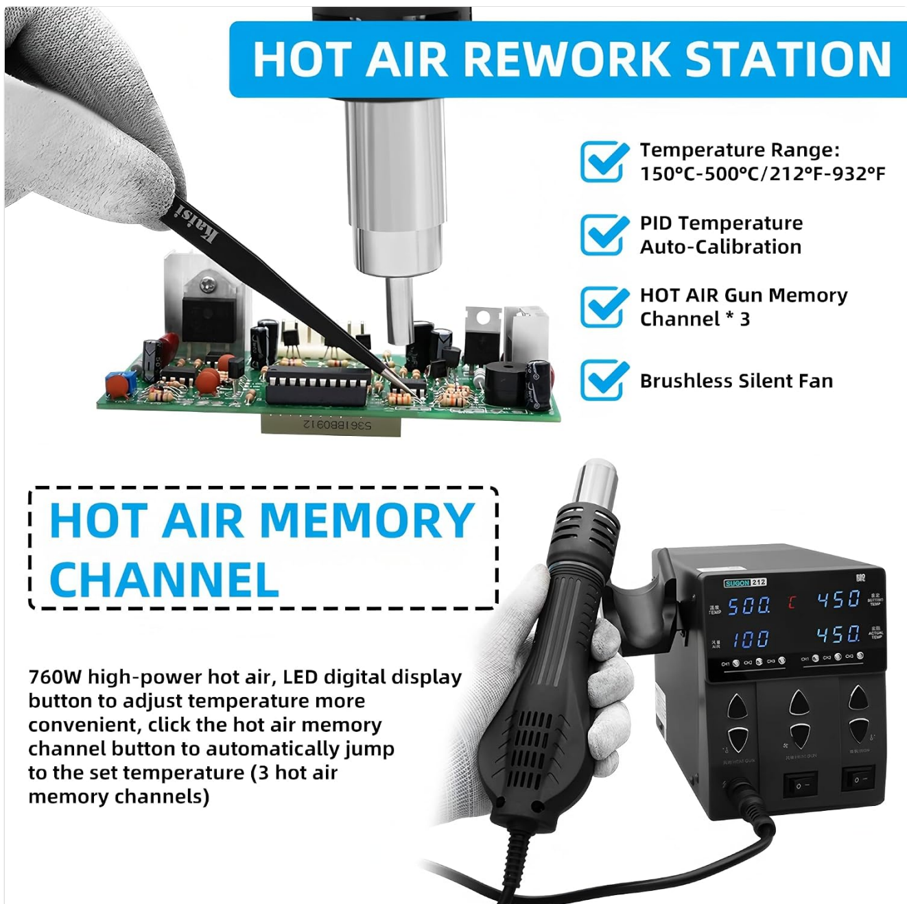
Image 6.2.1: Features of the hot air rework station, including temperature range, PID auto-calibration, memory channels, and brushless silent fan.
