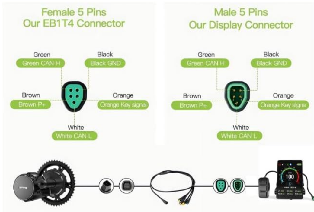
Figure 4.2: Detailed wiring diagram for the VD04 display cable, showing the female 5-pin 1T4 connector and the male 5-pin display connector with corresponding wire colors (Green CAN H, Black GND, Brown P+, Orange Key signal, White CAN L). An illustration shows the connection from the Bafang motor to the display via the 1T4 cable.
