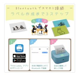
Turn on your Ninestar G&G Thermal Printer. Open the "Print-Label" app on your smartphone. Navigate to the connection settings within the app and select your printer (e.g., "GG-D220-XXXX") from the list of available Bluetooth devices to establish a connection.
