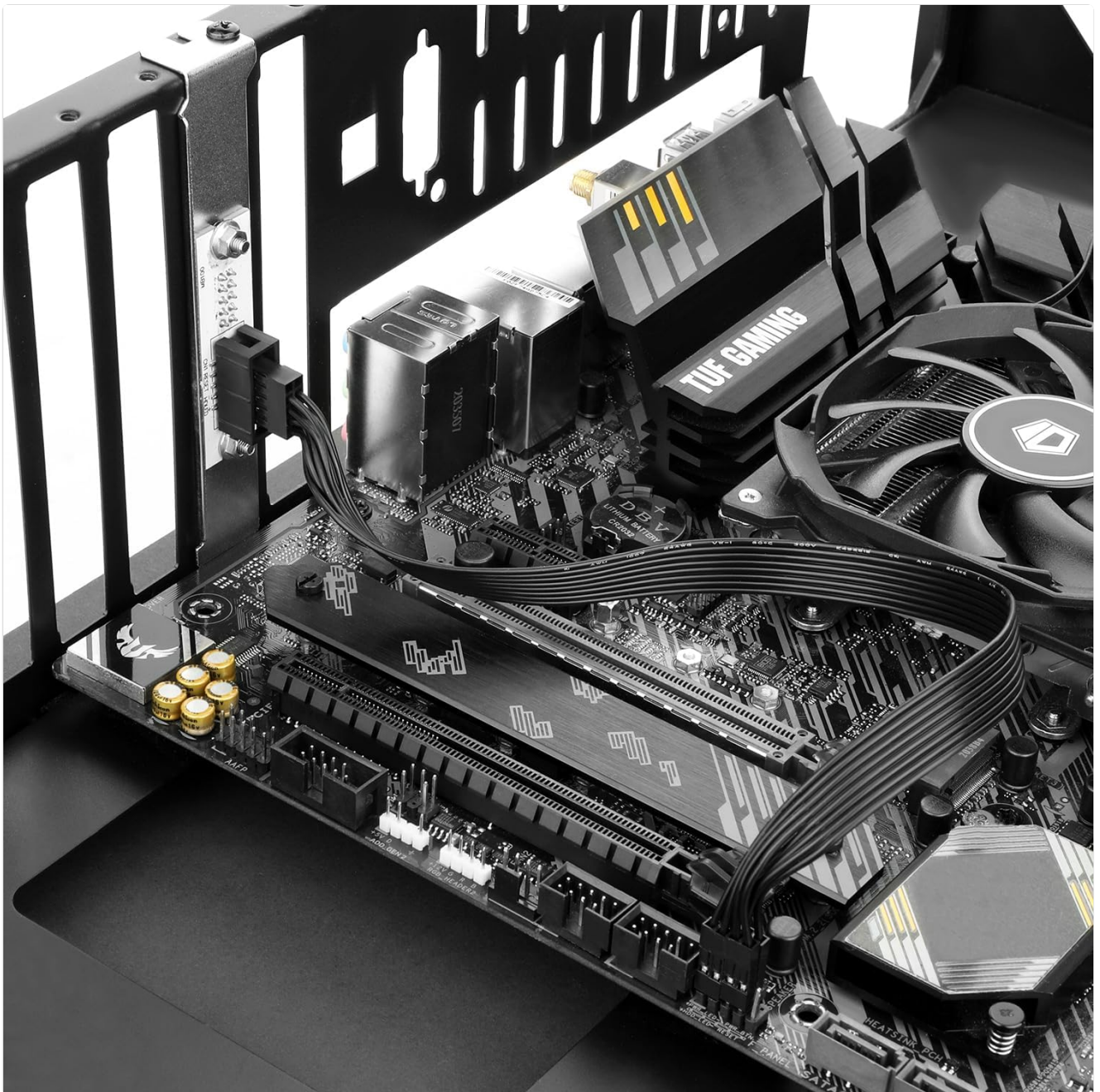
Image: The PCIe bracket is shown mounted in a PC case, secured with a screw. A motherboard is visible inside the case.
