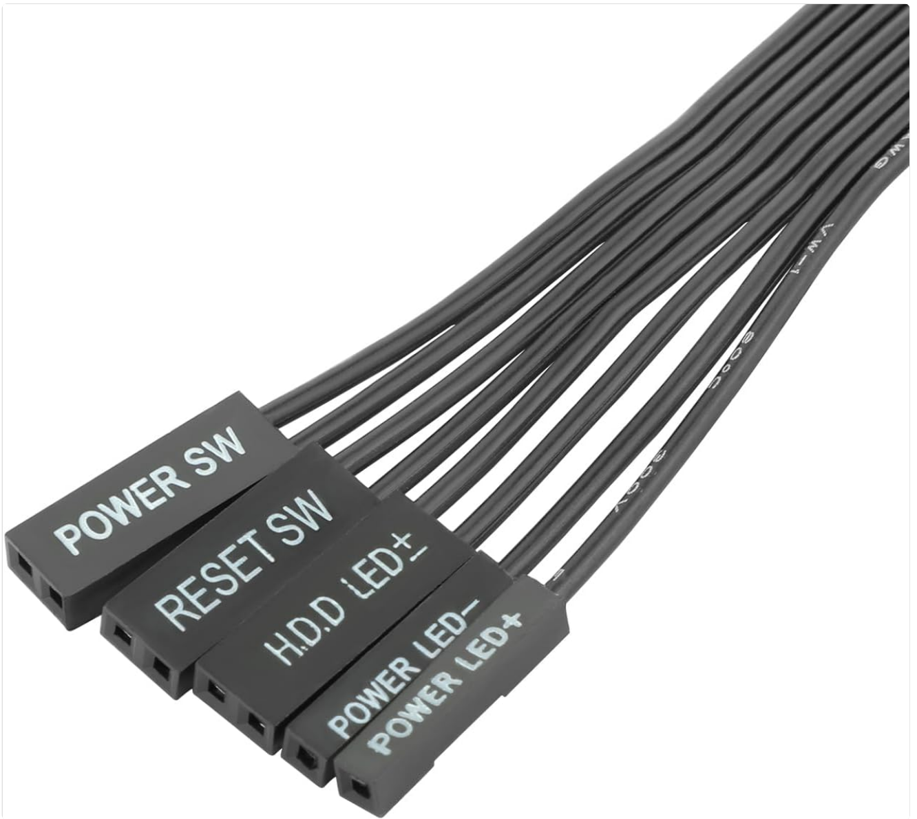
Image: A close-up view of the individual labeled connectors for Power SW, Reset SW, HDD LED, and Power LED, ready to be connected to the motherboard.
