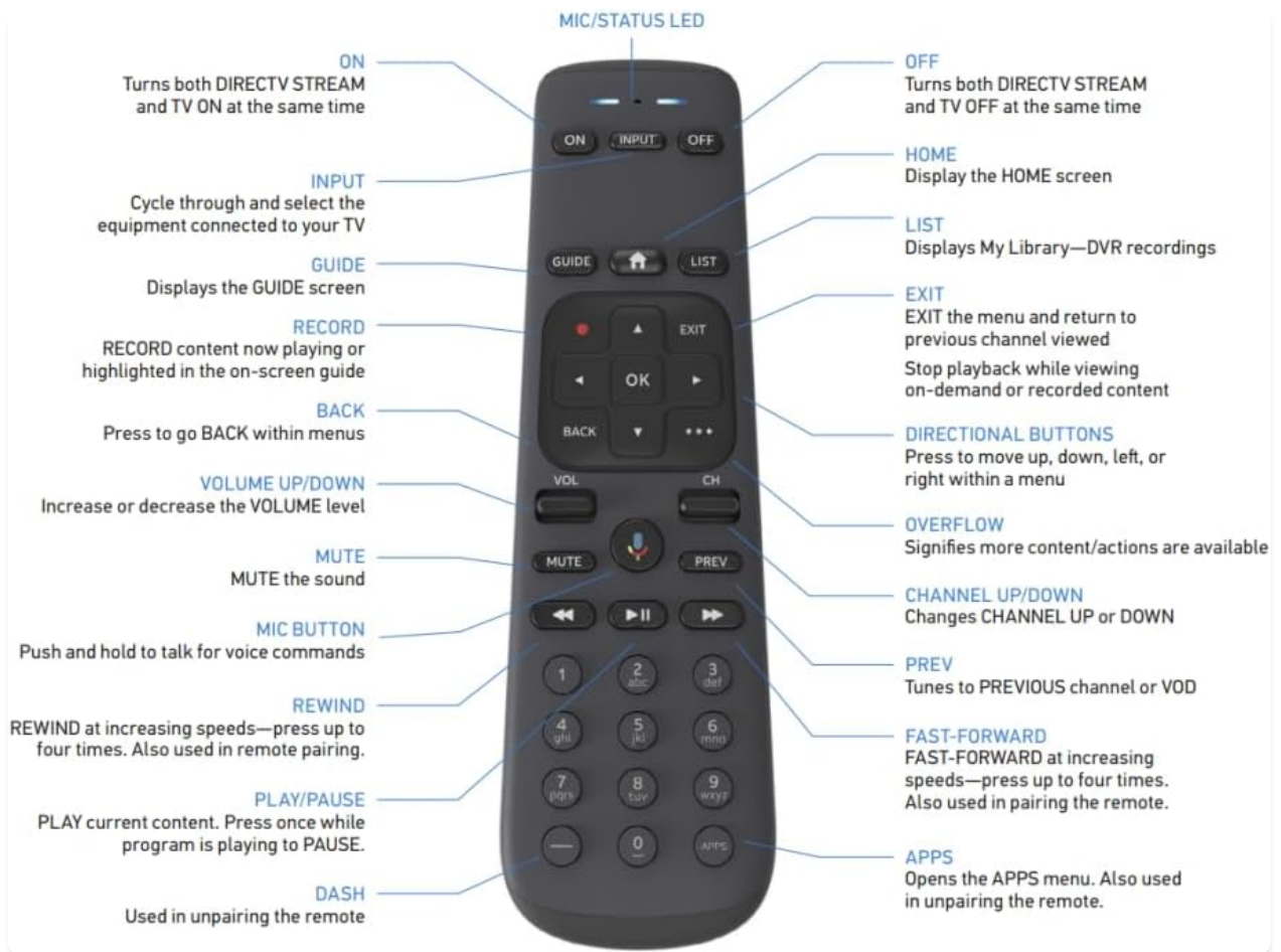
Image: Detailed diagram of the RC82V Remote Control with labels indicating the function of each button.
