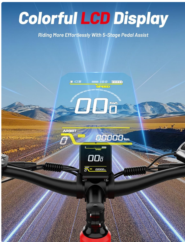
Figure 3.5: The colorful LCD display. This display provides real-time information such as speed, battery level, and pedal assist mode.
