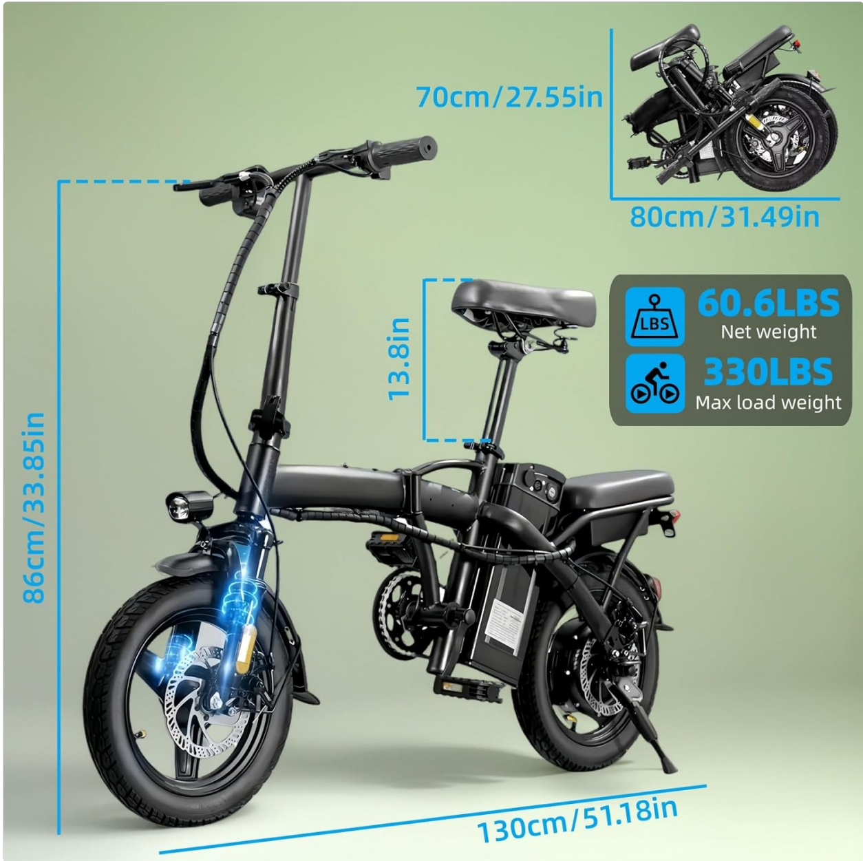
Image 8.1: Key dimensions and weight specifications of the electric bike.
