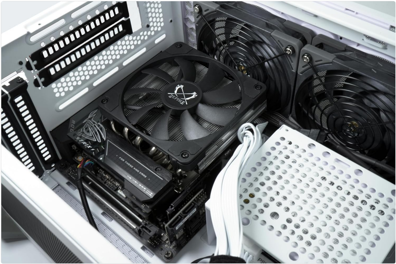
Image: The SCYTHE Big Shuriken 4 CPU Cooler installed inside a PC case, showing how it fits within a system's internal layout.
