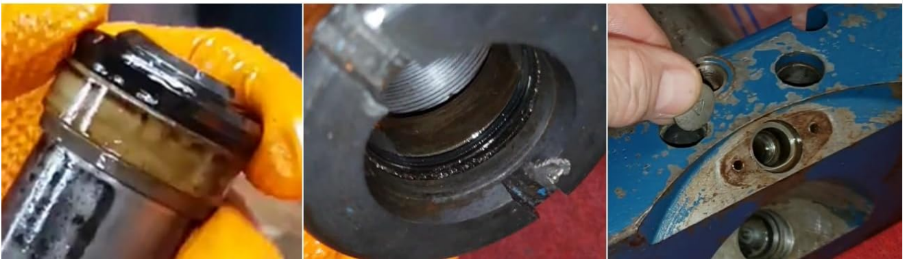
Image 4.2: Visual representation of a worn seal, the internal cylinder, and the process of installing a new seal.
