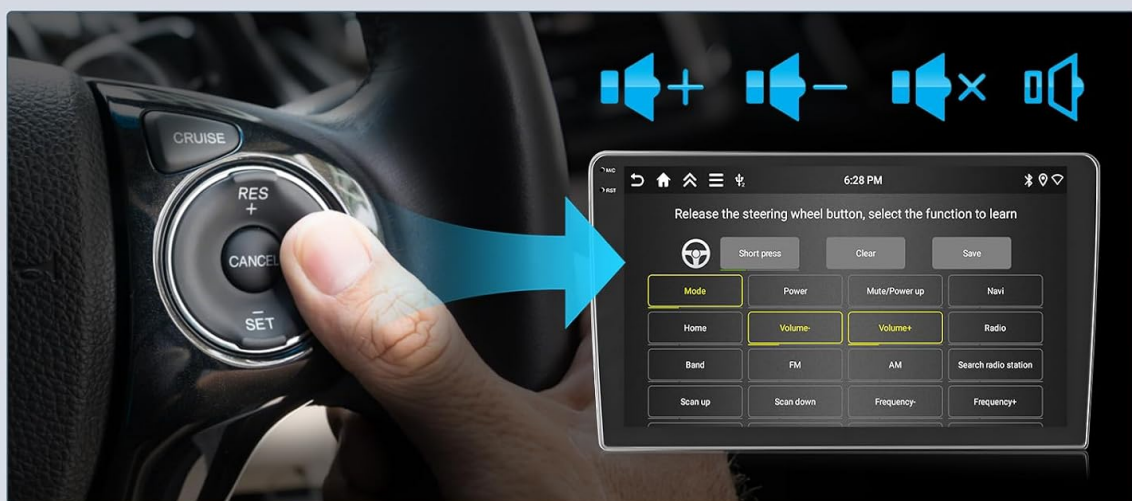
Image 6.4: Illustration of the Steering Wheel Control learning interface, showing how to assign functions to physical buttons, alongside a demonstration of the rear view camera display in both day and night vision.
