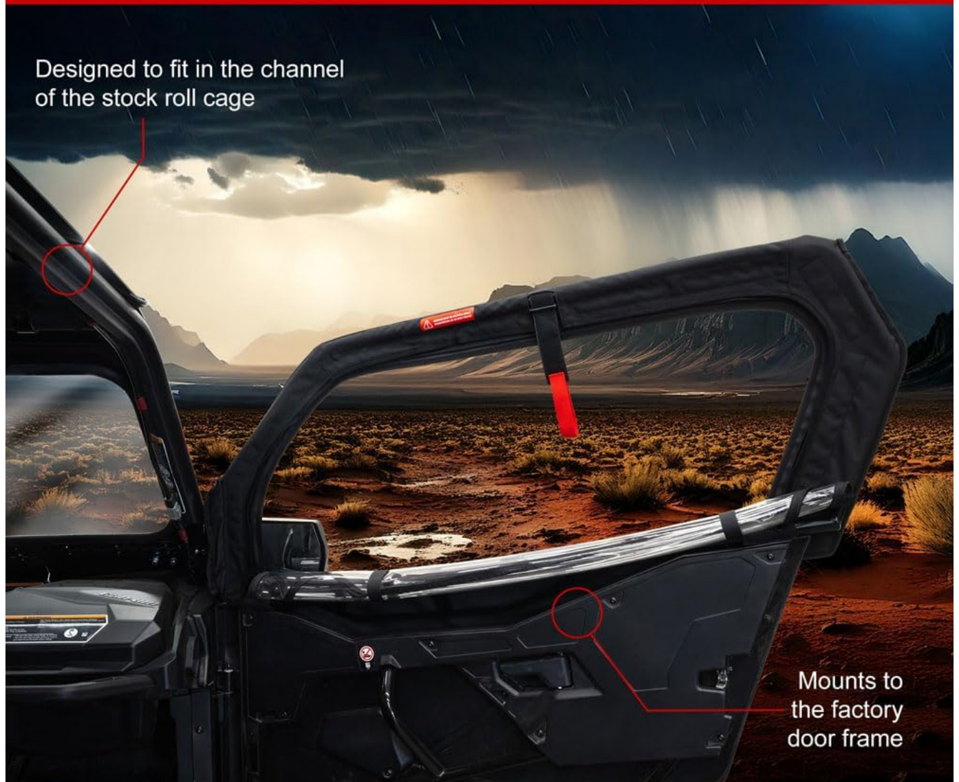
Image: Demonstrates the precise fit of the soft upper door to the UTV's roll cage and factory door frame.
