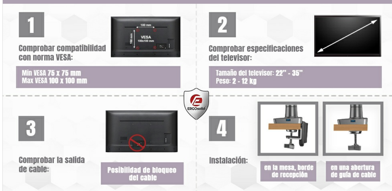
Figure 2: VESA compatibility and monitor specifications. This diagram illustrates the supported VESA patterns (75x75mm, 100x100mm) and the recommended monitor size and weight ranges for the arm.
