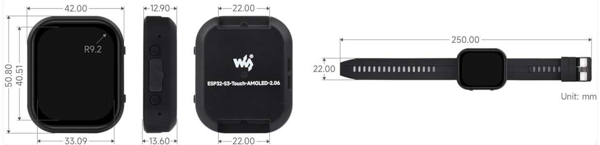
Figure 9: Outline Dimensions and Onboard Components
