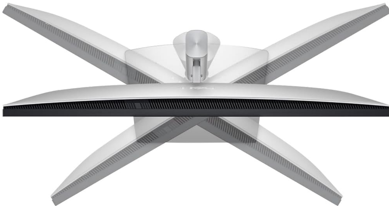
Figure 4.2: Monitor swivel adjustment.
