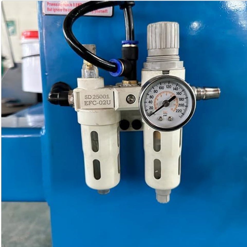
Image 2: Detail of the air filter and pressure gauge, essential for the pneumatic system's longevity.
