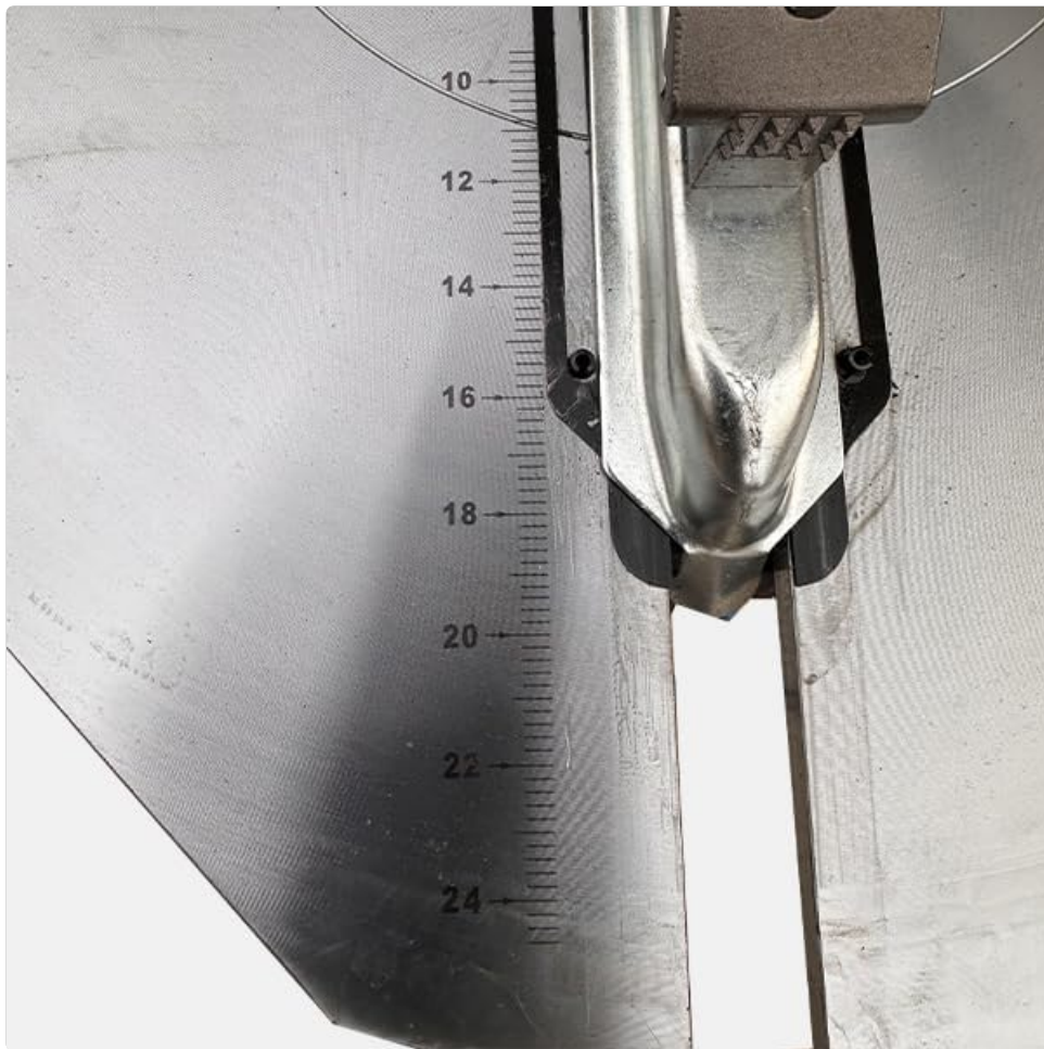
Image 9: The automatic measurement ruler, used for accurately inputting wheel dimensions for balancing.
