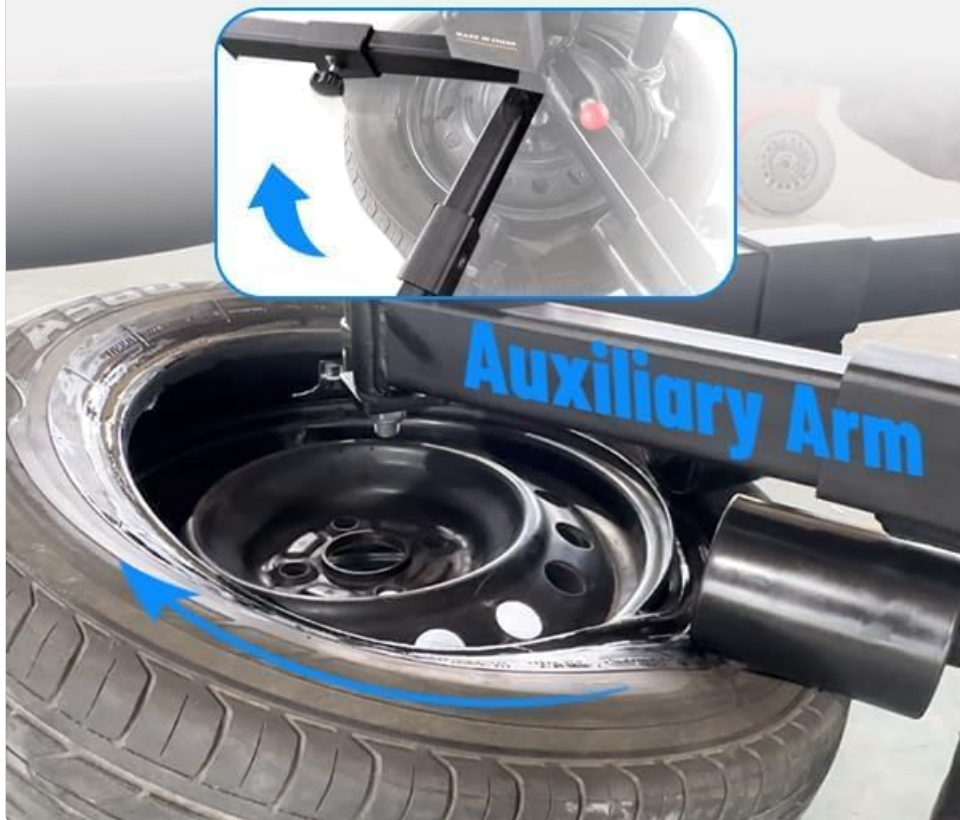
Image 4: The auxiliary assist arm in operation, demonstrating its function in removing tires with ease.
