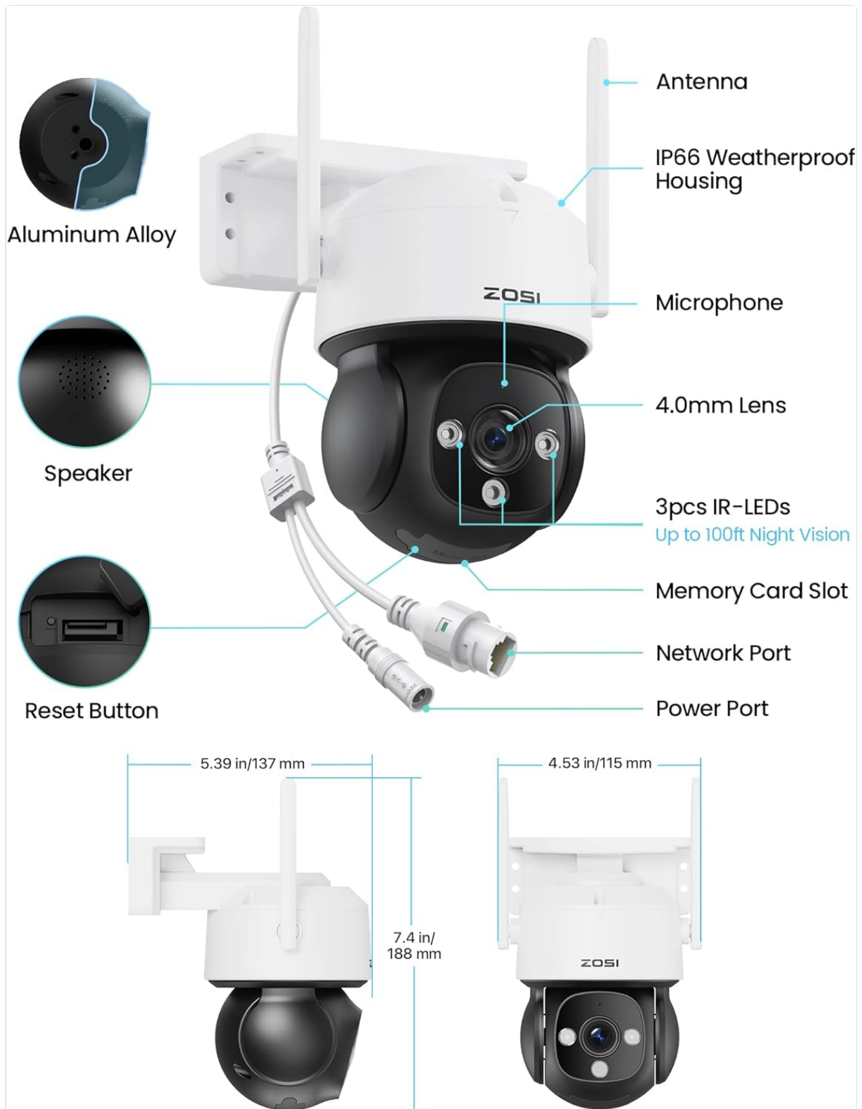
Image: Labeled diagram of the ZOSI C290 camera components.
