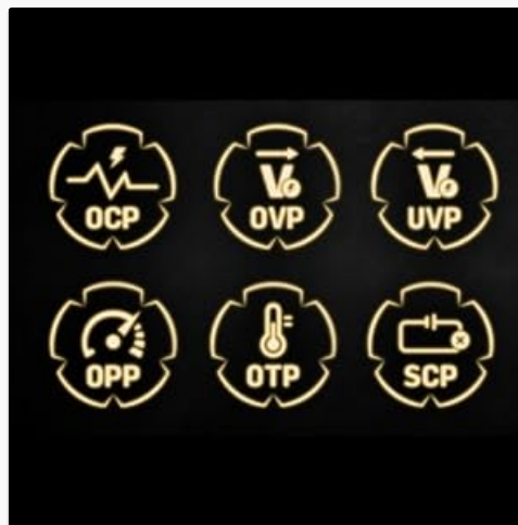
Image 4.4: Multiple protection circuitries for system safety.
