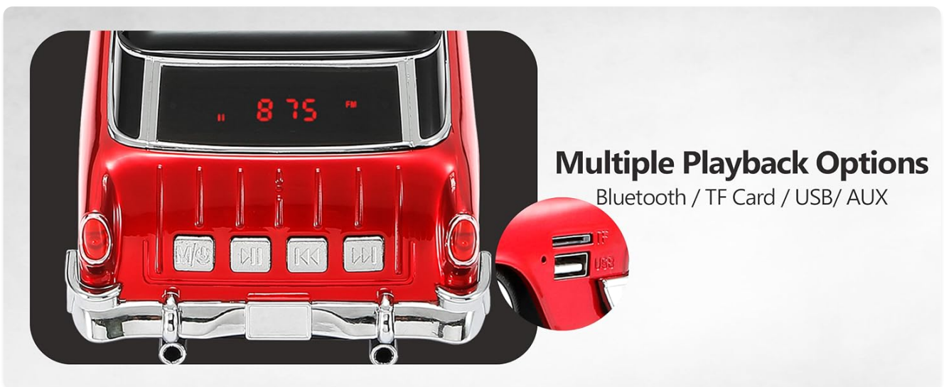
Image: Close-up of the speaker's rear, highlighting the USB and TF card input ports.
