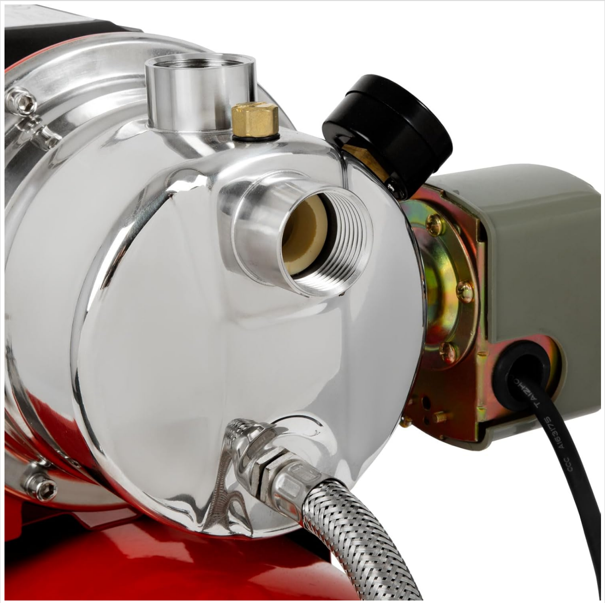
Figure 5: Close-up of the pump's water inlet (1" internal thread) and outlet (0.5" internal thread) connections, along with the flexible hose connecting to the pressure tank.
