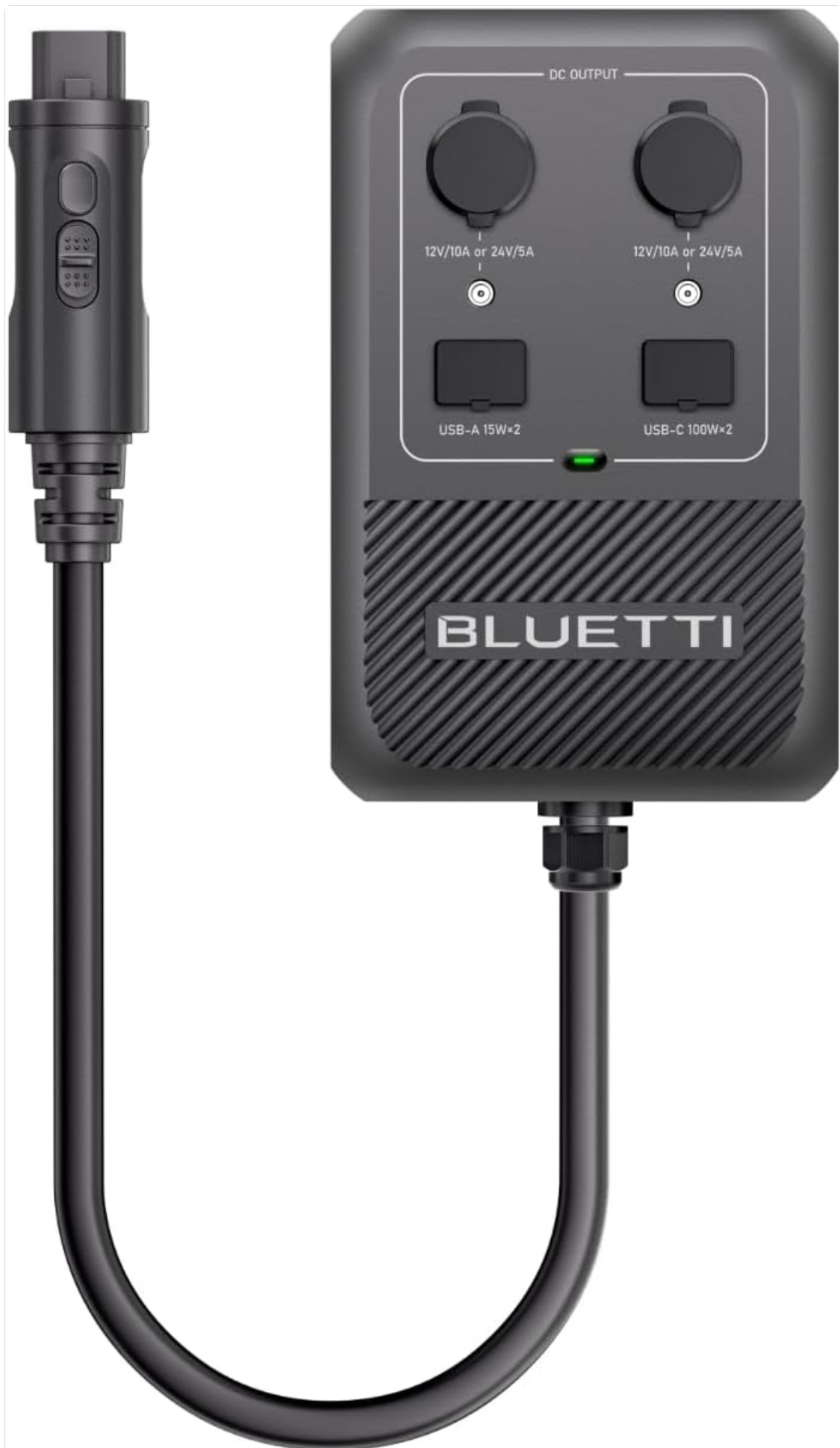
This image displays the BLUETTI HUB D1, a compact grey unit featuring two 12V/10A or 24V/5A DC output ports (cigarette lighter style), two USB-A 15W ports, and two USB-C 100W ports. An on/off switch with a green/blue indicator for 12V/24V selection is also visible. A cable with a P090D connector extends from the bottom, designed for connection to compatible BLUETTI power stations.
