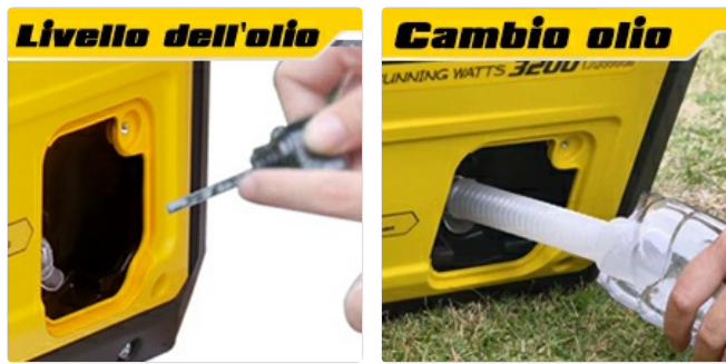
Figure 4.1: Oil Level Check and Funnel. Ensure oil is at the correct level using the dipstick and use the funnel for clean filling.
