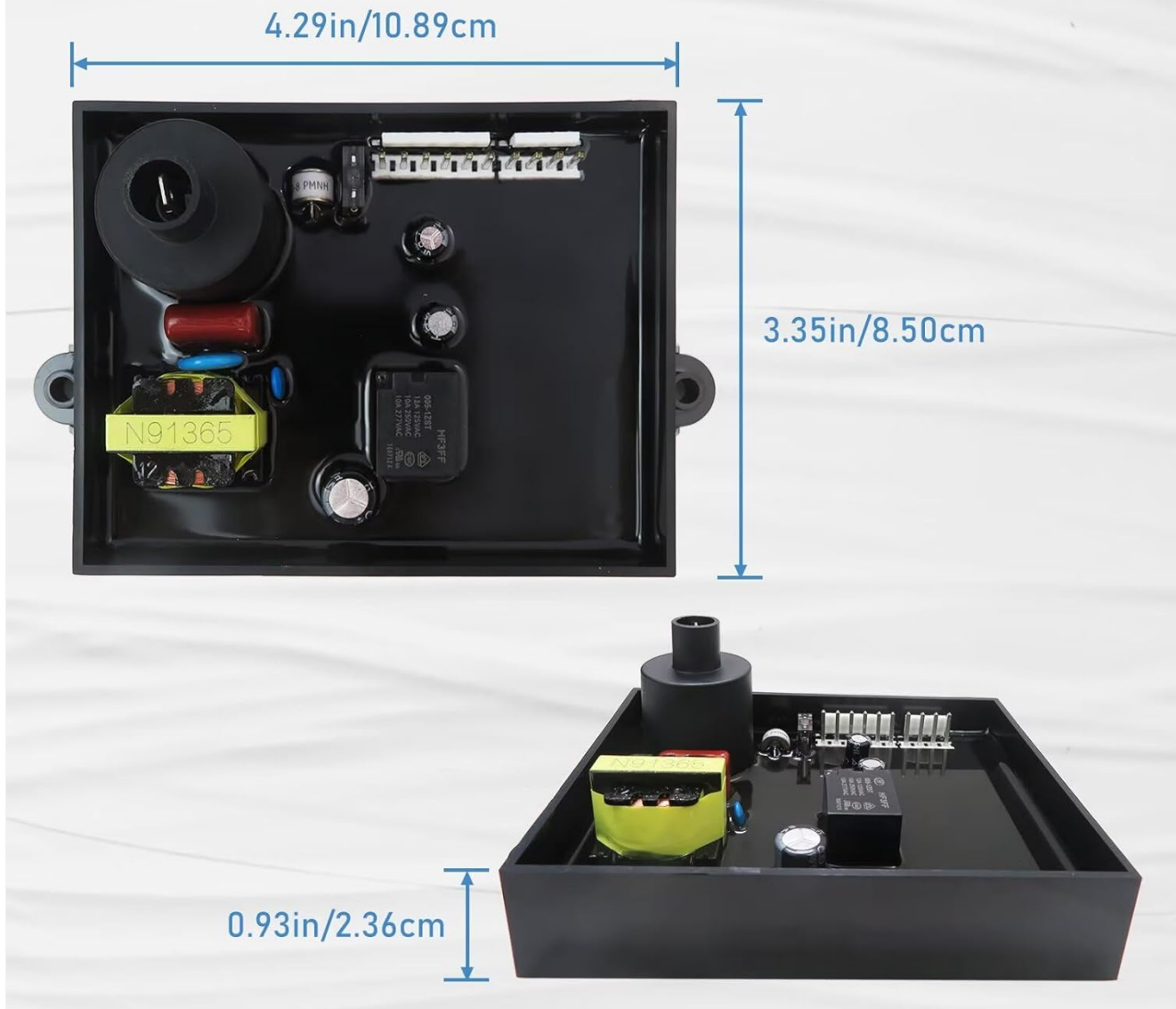
Figure 6: Dimensions of the 91365 RV Water Heater Control Circuit Board.
