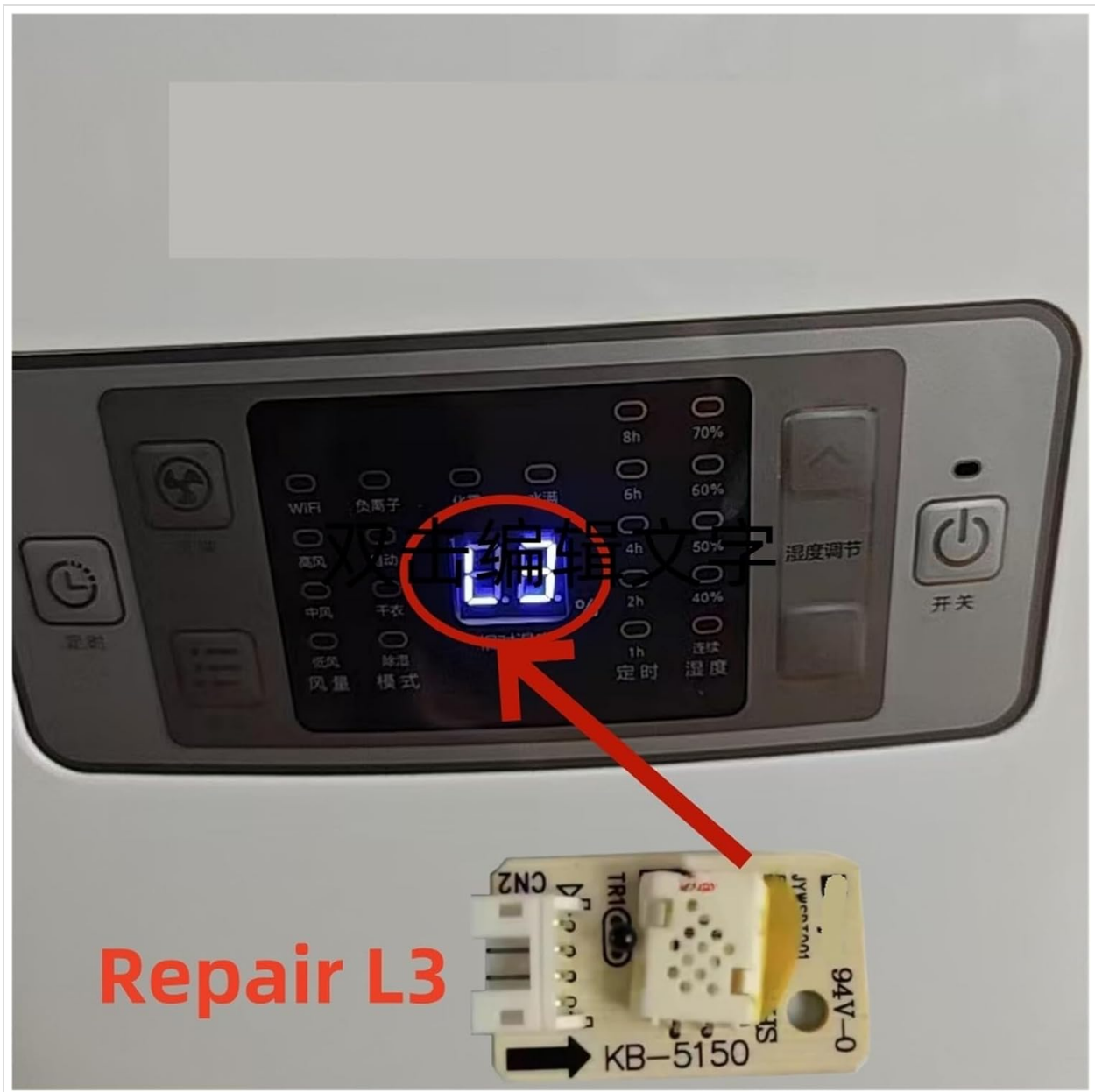
Figure 3.1: KB-5150 Sensor connected to a dehumidifier control panel. This image illustrates the sensor's integration into a dehumidifier system, indicating its repair or replacement context.
