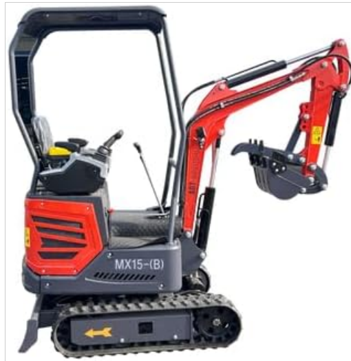
Figure 2.1: Side view of the AGT-MX15-(B) Small Excavator, showing the main body, tracks, and boom assembly.
