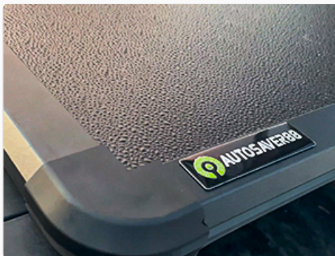
Image: Detail of the weather strip, designed to prevent elements like rain and dust from entering the truck bed. Regular inspection of this seal is crucial for maintaining protection.
