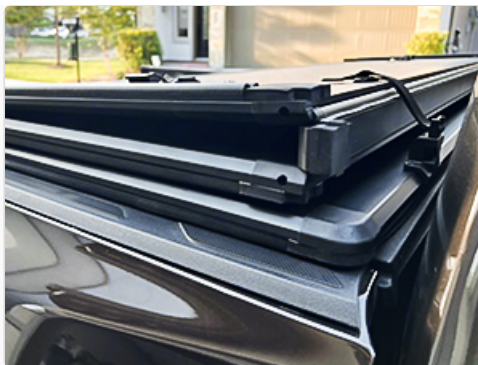
Image: Detail of the nylon buckle system, which is used to securely hold the tonneau cover in its folded position against the truck cab.
