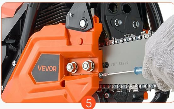
Close the side cover, adjust the chain tension, and ensure the distance between the chain bottom and guide bar is 2-4 mm
