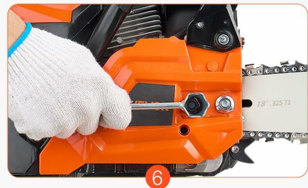
Install the chainsaw, ensuring the direction of the teeth is correct
