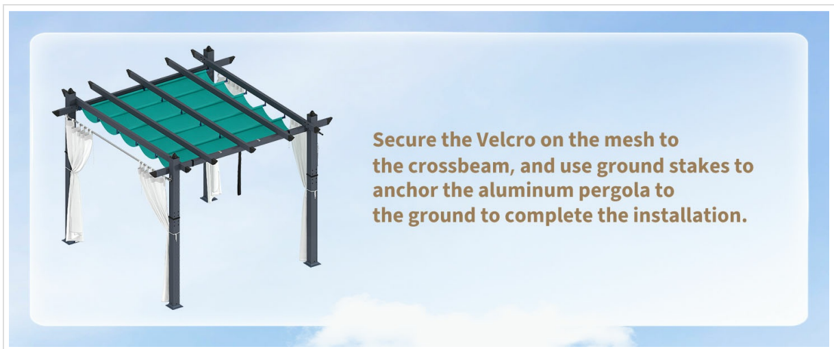
Image: A diagram showing the final steps of assembly: securing the Velcro on the mesh to the crossbeam and using ground stakes to anchor the aluminum pergola to the ground.
